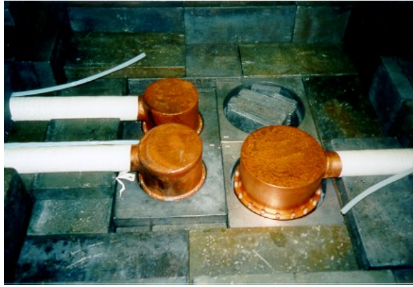
Figure 2.1: A detail of the IGEX shielding in preparation. There are two detectors of 0.7 kg each and one of 2 kg inside the Marinellis lead.
