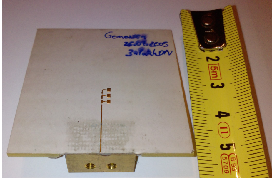
Figura 6-36 Circuit measuring the Antenna Parameters of the 1x3 Patch Array without Phase Shifts
