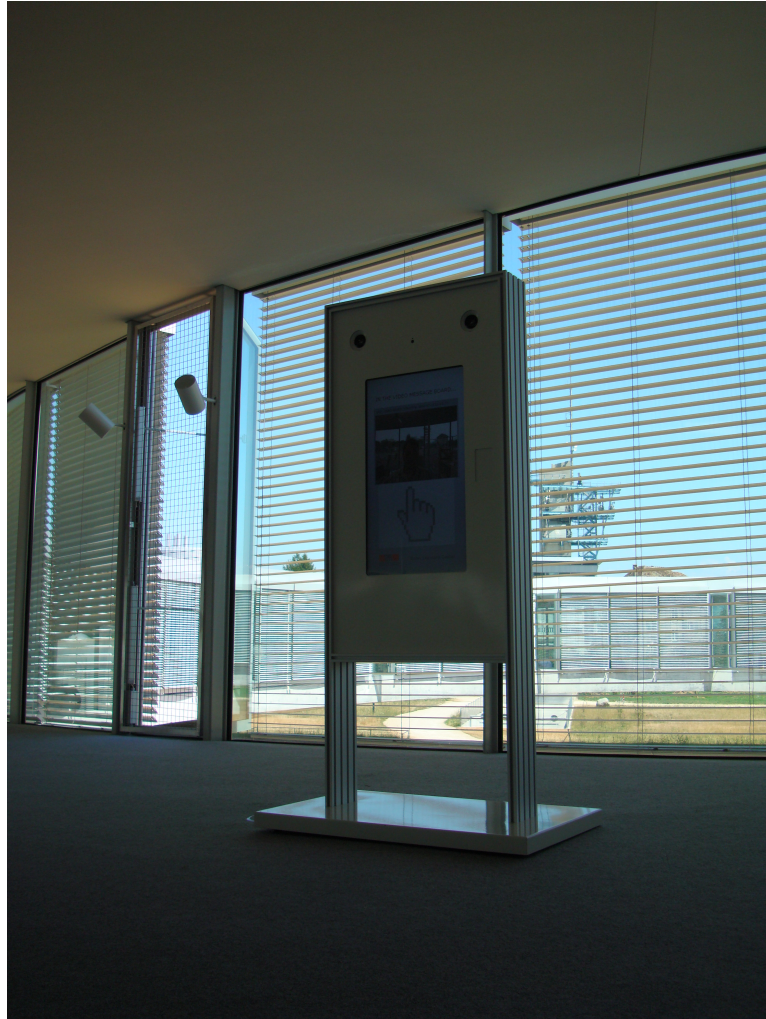
Figure 4.2: Final built and working prototype of the Interactive Kiosk for the Rolex Learning Center
