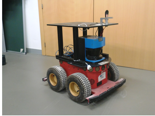
(b) The tele-operated Pioneer 3-AT robot
