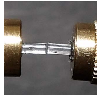
Figura 75 Desalineamiento angular Axis Pitch .
