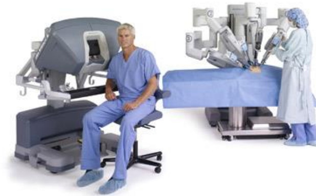
Figure 1.1: Master and slave devices of Da Vinci Surgical System [3]
