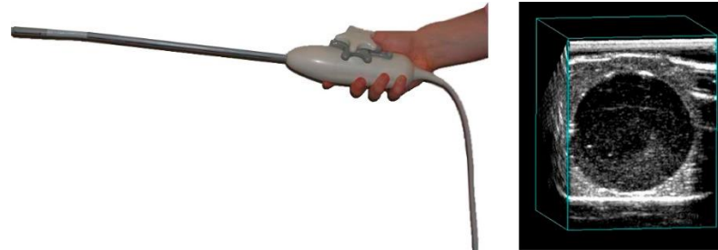
Figure 1.5: Ultrasound-based sensor and 3D image
