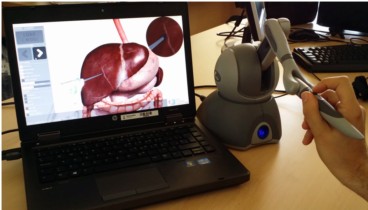
Figure 1.3. Appearance of the computer-based surgical simulator developed at Universidad de Zaragoza, consisting of a laptop (left), and the stylus-based haptic interface Phantom Omni by GeoMagic SensAble (right).
