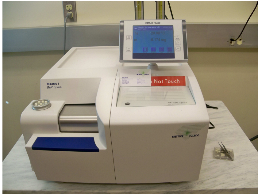
Figura III.1: Equipo TGA Mettler Toledo TGA/DSC 1 Star e System
