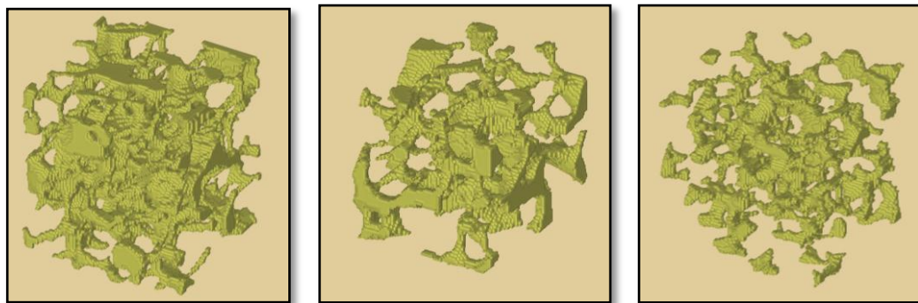
Figure 16: Creation of voxel mesh for specimen #30 (on the right), specimen #20 (in the middle) and specimen #15 (on the left) using the Voxel Create Mesh Module
