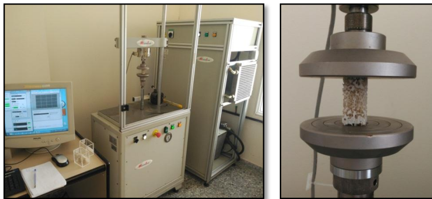
Figure 11: On the left, servo-hydraulic material testing machine; on the right, uniaxial compression test
