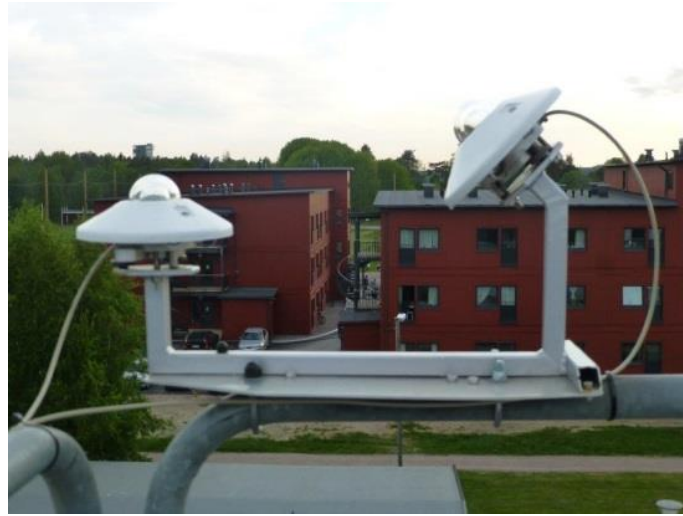
Fig 3.2. Pyranometers number 1 and number 2 placed on the laboratory system.
