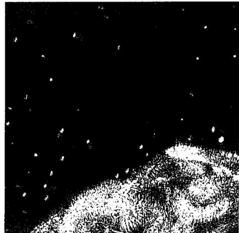
FIGURE 4: Perturbed liquid surface, and atomized droplets. Field of view of 1.5 x 1.5 mm and a resolution of 2  $\mu\text{m}/\text{pixel}$ . Forcing voltage of 37 V
