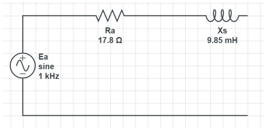
Figure 30: Equivalent circuit of 'a' phase
