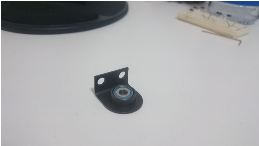
Figure 21: Housing and bearing used in the prototype, model PF-5M
