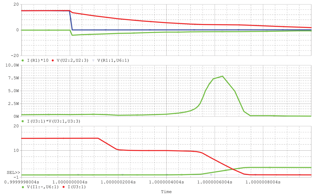
Figure 6.7.: Simulation without snubber. Top: gate current (Green, 10:1), input voltage (Blue), gate-to-source voltage (Red). Centre: power dissipated by a single MOSFET. Right: drain-to-source voltage (Green), drain current (Red)
