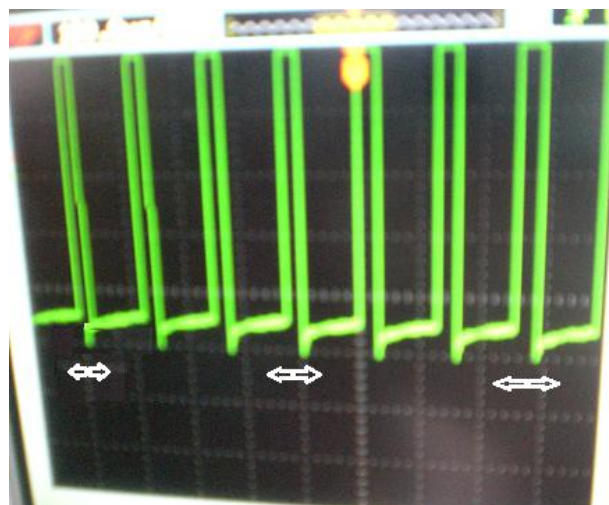
Figure 28. The duty cycle is increasing in one period.
