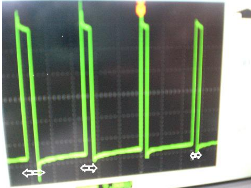
Figure 29. The duty cycle is decreasing in one period.
