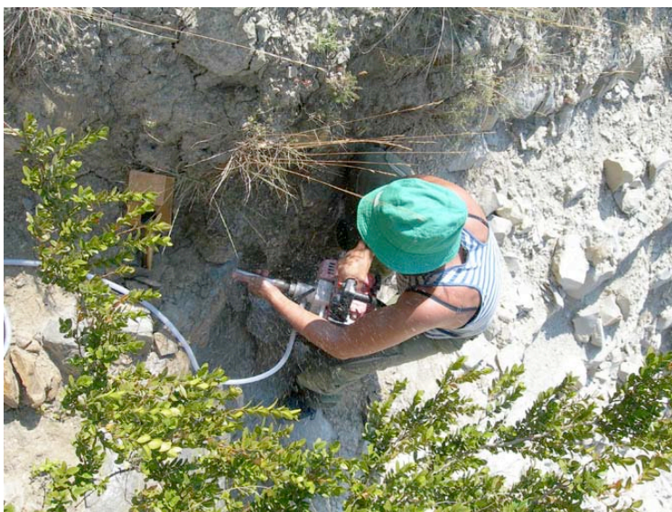
Figure 2. Fieldwork; drilling and orientation of paleomagnetic samples
