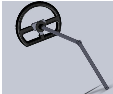
Figure 35'. Assembly steering wheel-quick disconnect-steering column
