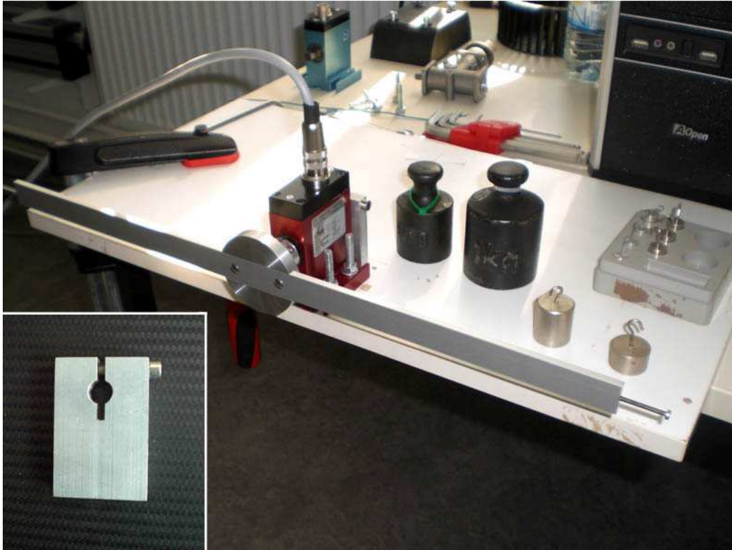
Figure 2.5: Pre-calibration set for the torque sensor
