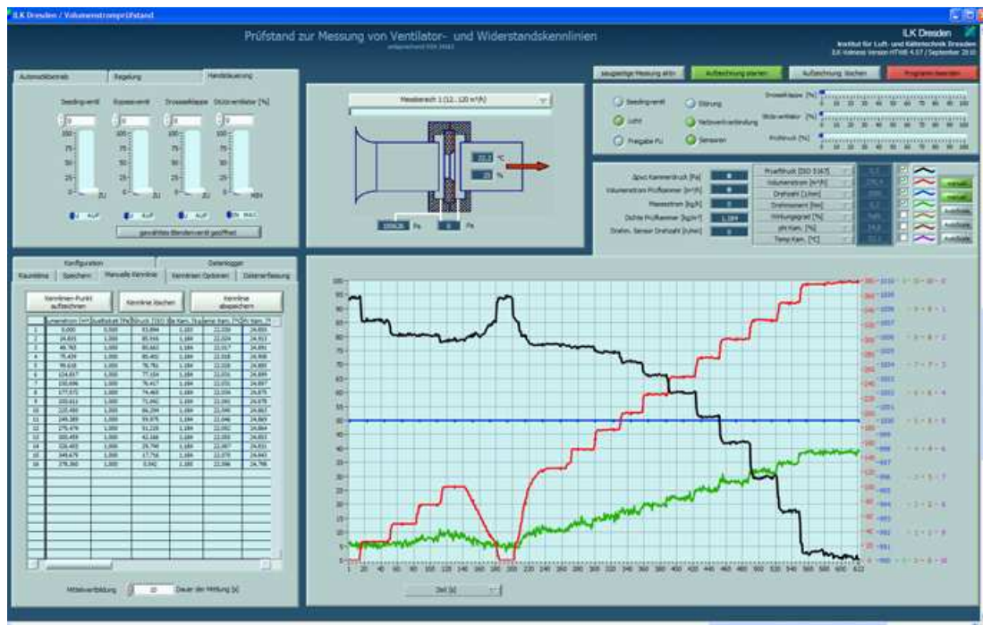
Figure 6.3: Front panel of the software used to control the test chamber
