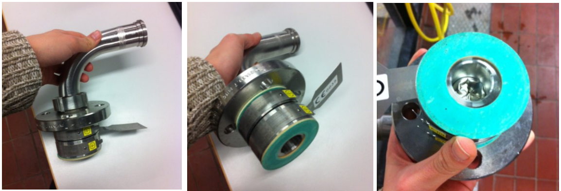
Figure 11. Dismantled rupture disk.
