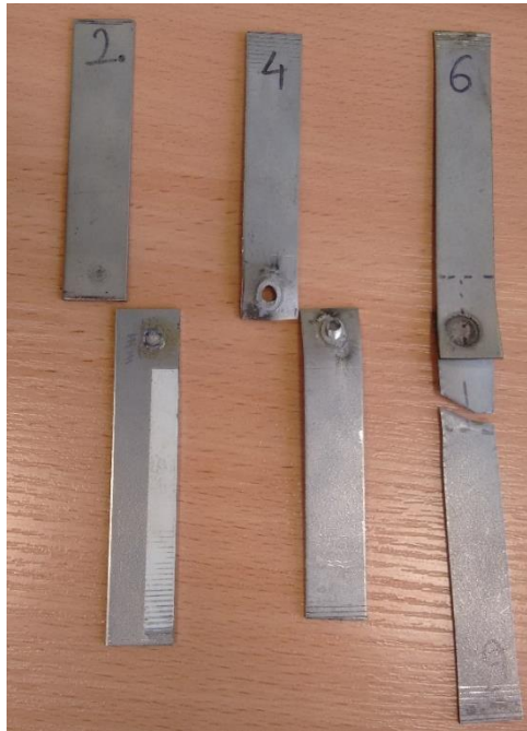
Figure 8.9 Spot Resistance specimens after Tensile Strength Test
