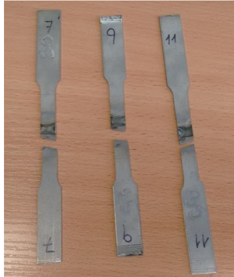
Figure 8.1 Micro Plasma specimens after Tensile Strength Test
