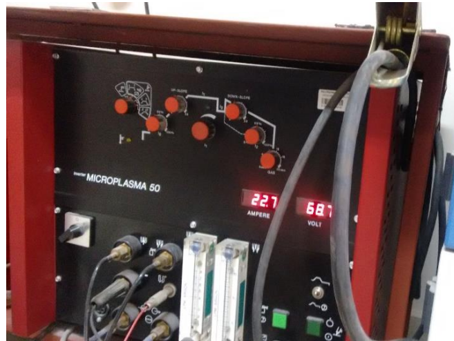
Figure 6.2 Micro Plasma machine. Amperage and Voltage
