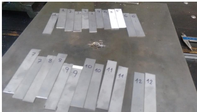
Figure 7.10 Samples ready to be welded
