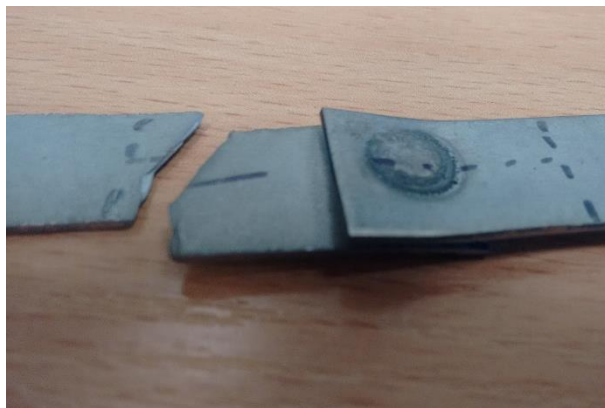
Figure 8.18 Detail of the rupture of the test piece 6
