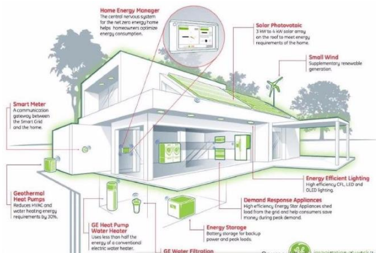
Figura 6. “Esquema” de un BEMS (neZEH, Nearly Zero Energy Hotels).
