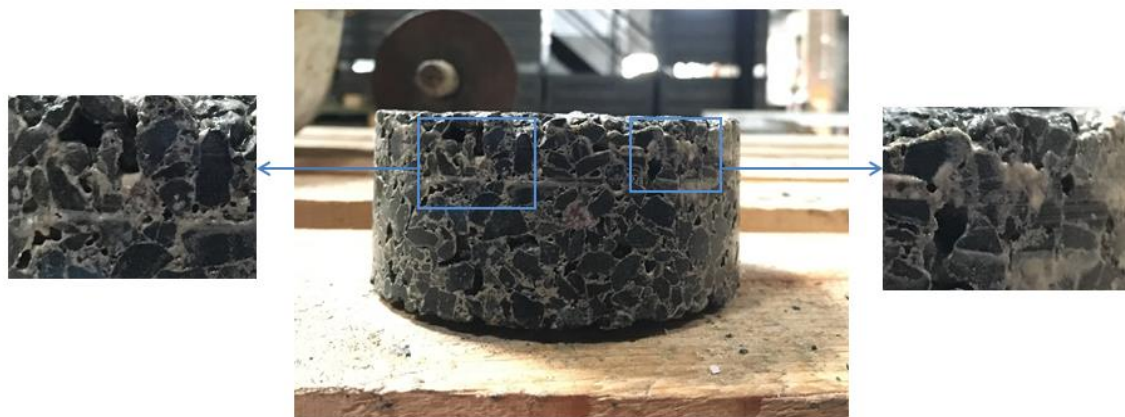
Figure 13: Accumulations of particle matter inside the pores of the clogged specimen with grain size distribution PA8.
