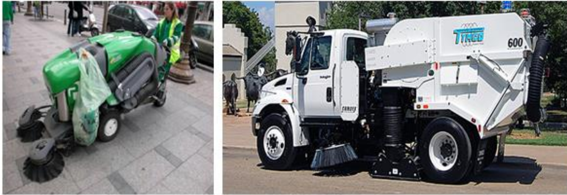
Figure 4: Mechanical street sweeper (left) and vacuum sweeper (right).
