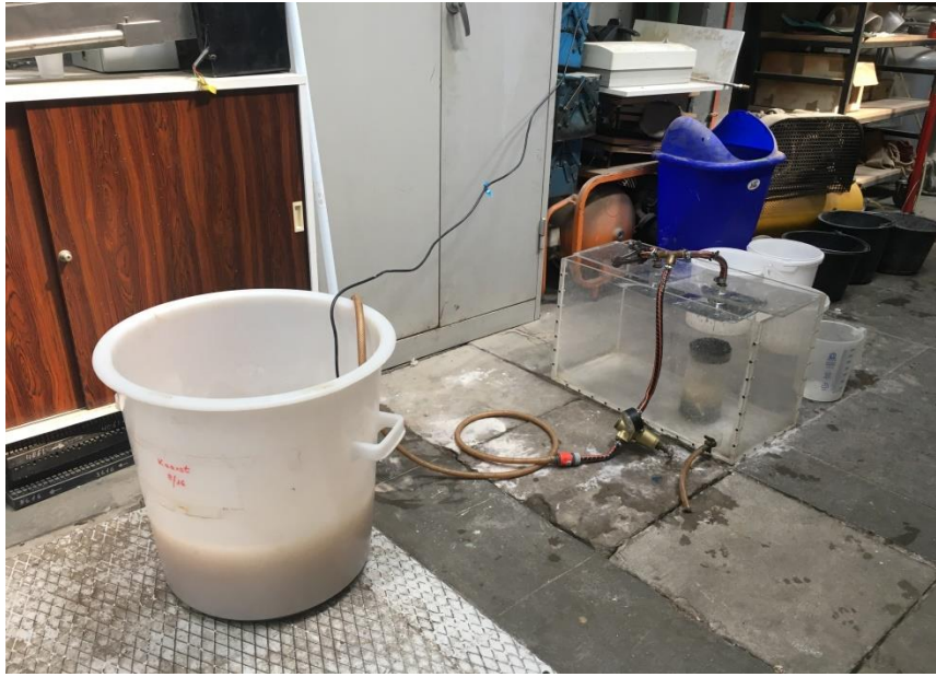
Figure 8: Final building of the filtration experiment. L-R: Influent container, pump, overflow and effluent containers (with specimen), and several recipients for keeping the effluent samples.
