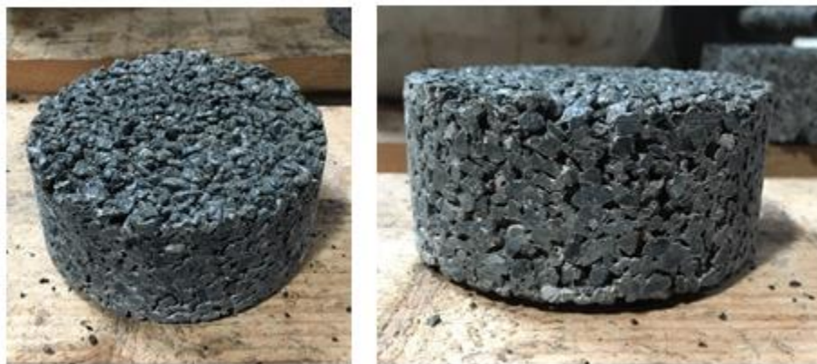
Figure 11: Tested PU-bonded pavement specimen with grain size distribution PA5.
