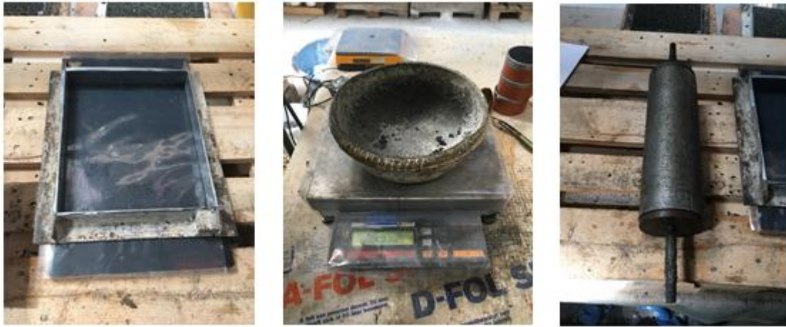
Figure 5: Material used for the production of specimens. L-R: Mold covered with adhesive tape, weight and bucket where the aggregates are mixed with the polyurethane, hand roller.
