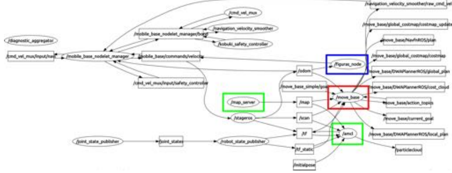
Fig. 6. Diagram of the main ROS modules used in our system.
