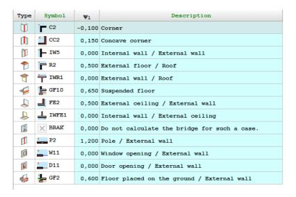
Entering in details in, for example, the first thermal bridge:
