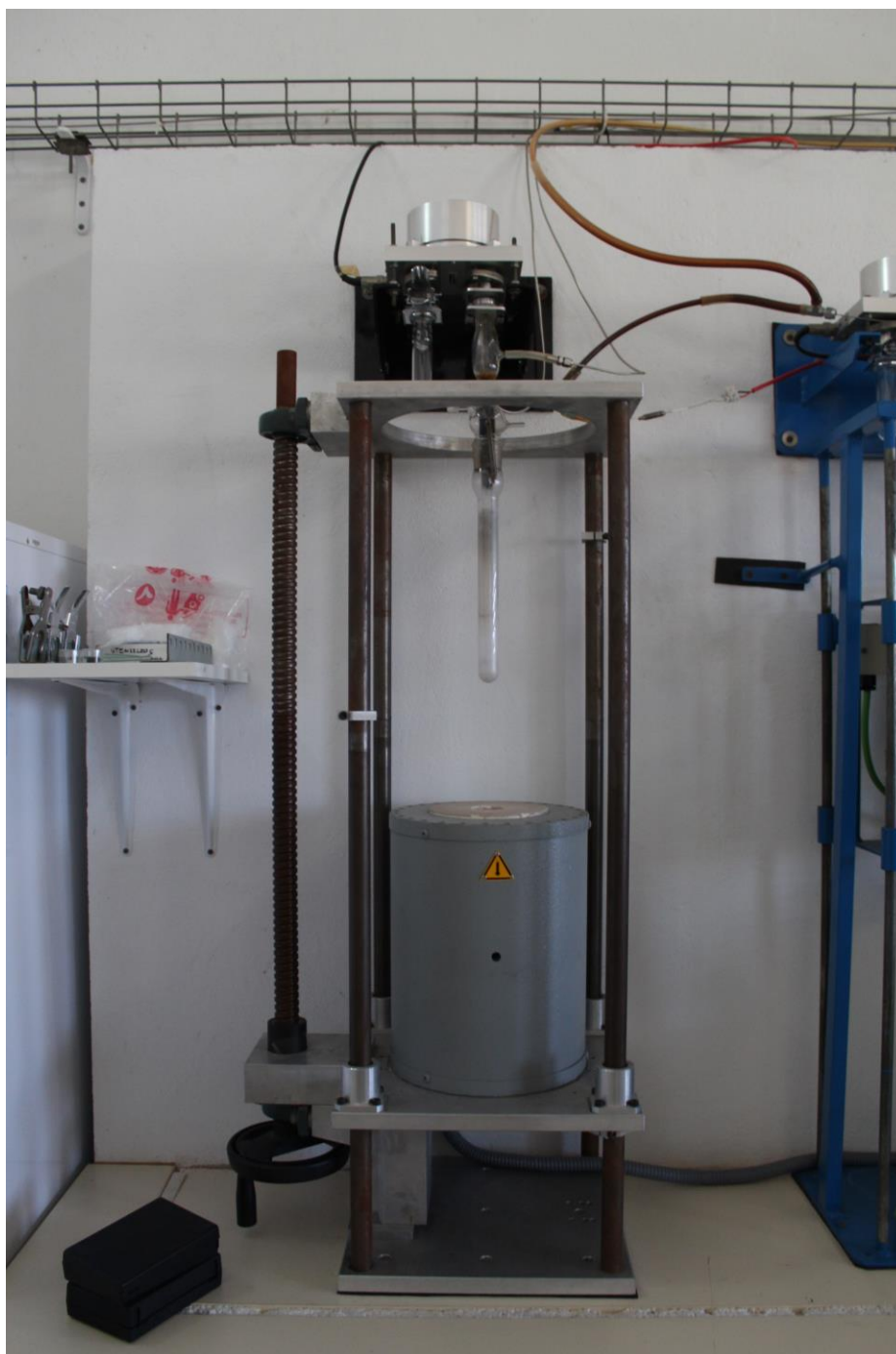
Figura I.5. Termobalanza CI Electronics MK2
