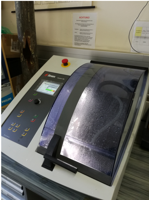
(7) Disc cutting machine with horizontal axis cutting precisely along the weld line for obtaining an accurate longitudinal sample from one of the weld plates
