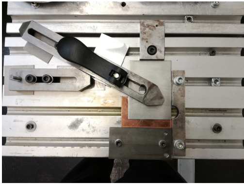
(1) Picture that shows how the Samples are placed in the fixation system
