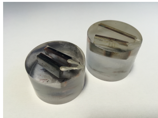
(6) Final aspect of the mounted samples No. 1 & 7 after EDX measurements. It can be appreciated the thin dark film on the upper surface of Au-Pd and the electric path towards the bottom part. They were mounted in order to be seen the seams from the lateral surface
