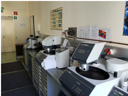
(3) In the background the mounting press for generation of the mounting samples and in the foreground two disc polishing machines with suitable supports for the mounted samples
