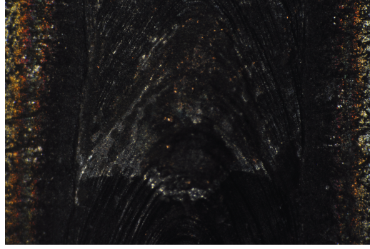
Figure 4.5: Image of one hump, it can be appreciated the drastic change of the seam appearance. These periodical humps were distanced approximately 5 mm one each other in sample No. 3
