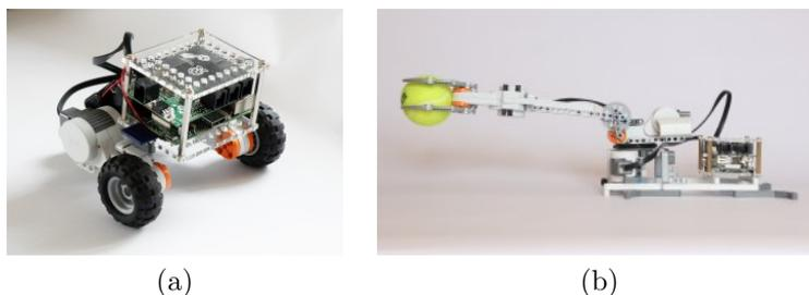
Figura 1.2: (a) Robot de control remoto con Raspberry Pi. (b) Brazo robótico con Raspberry Pi. (Fuente [www.dexterindustries.com/BrickPi](http://www.dexterindustries.com/BrickPi))
