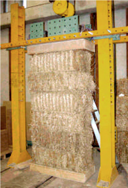
06. Test de compresión Peter Walker Dept. Architecture & Civil Engineering University of Bath (2004)
