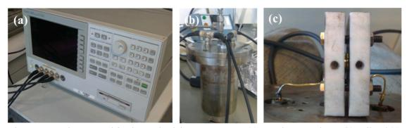
Figure 3.7. Equipment used for the conductivity measurement: (a) Impedance Analyzer, (b) Cell and (c) Conductivity module with gold electrodes.
