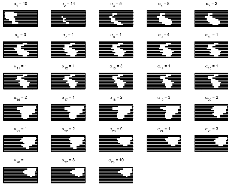
(a) ONS segmentation with 28 segments and 126 MU when r = 23 and d \leq 2 .
