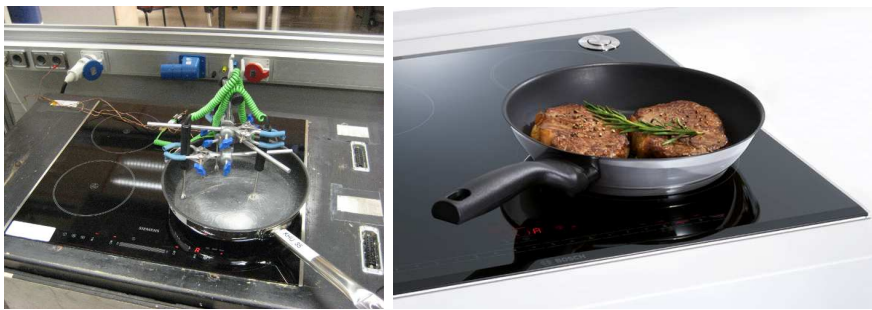
Figure 8.11: Domestic Induction hob used during verification tests with three thermocouples to measure the temperature of the cooking pot (left). Final system in household conditions (right).
