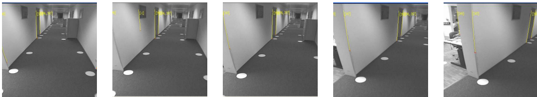
Figure 8.18: An example of the images used by the 9 robots during the navigation to test the proposed method [60]. Although the data set also provides artificial landmarks (white circles on the floor), we test the algorithm using the lines extracted from natural landmarks (in yellow).
