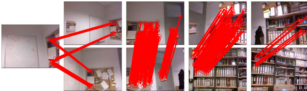
Figure 8.25: Images taken from the first robot poses. We are depicting the matches (red lines) between some of the images.
