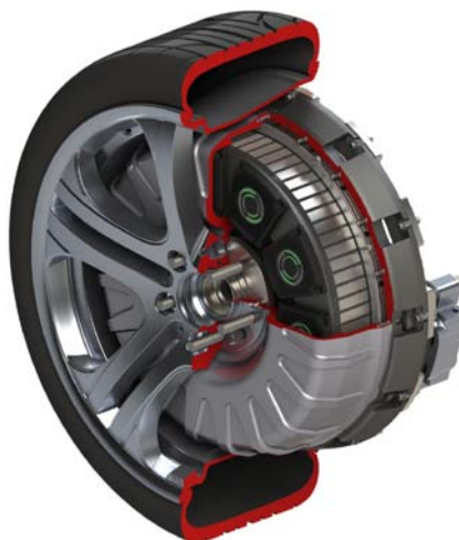
Figura 23. Motor rueda Protean Electric PD18 (9)
