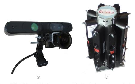
**FIGURE 3.13.** (a) Fisheye with RGB-D camera system. (b) Omnidirectional camera rig composed by 8 Asus Xtion Pro Live arranged to achieve 360 degree field of view.
