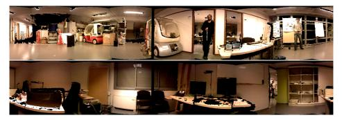
**FIGURE 3.15.** Panoramic views from two different scenes obtained with the 8 RGB-D camera rig. The views have been obtained by reprojecting the 3D points transformed to a common reference frame with the relative poses obtained following our multi-camera calibration method.
