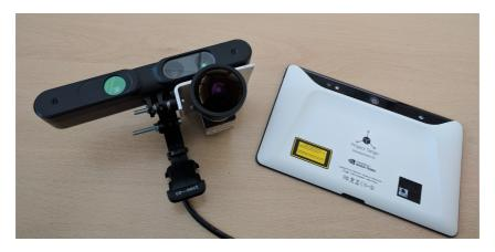
**FIGURE 4.14.** The two devices used to collect the data for our experiments. On the left, an RGB-D camera (ASUS Xtion Pro Live) with an adjacent fisheye camera. On the right, the Google Tango Development Kit.
