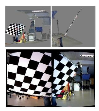
**FIGURE 3.14.** *Above*: Visual evaluation of the RGB to depth camera calibration with a checkerboard with the point clouds reprojected to a common reference frame (general and lateral views). *Below*: a panoramic reprojection of the 3D points where we can see the checkerboard's pattern continuity.
