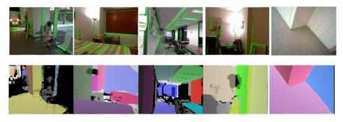
**FIGURE 3.10.** Examples of common indoor scenes used for calibration, like wall-wall and wall-ceil junctions. The first row shows the RGB images with the lines extracted in green. The second row shows the corresponding depth images with the planar surfaces colored in different colors. Images (1-4) belong to the NYU2 RGB-D dataset [Silberman et al., 2012].
