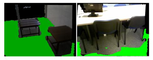
FIGURE 2.11. In green, the portion of the ground which can be walked over as it has no obstacles.
