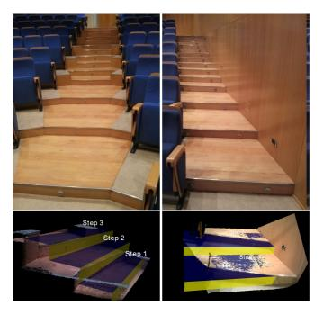
**FIGURE 2.23.** Two examples of complex stairs where the modeling fails because of atypical shapes (left) or non-Manhattan directions of the edges with respect to the wall (right).
