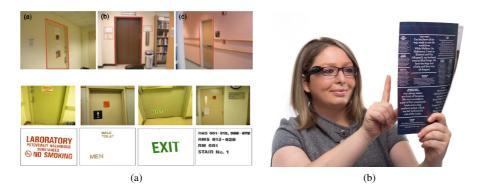
**FIGURE 1.2.** (a) Example of door detection and text information extraction with conventional cameras from [Tian et al., 2013]. (b) A woman using OrCam, a commercial visually impaired aid attached to the glasses that using a camera performs tasks such as reading text aloud.
