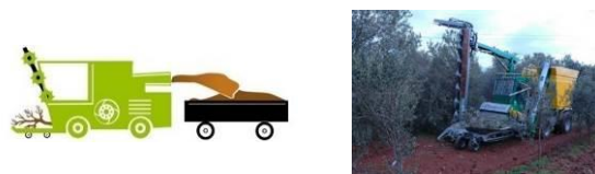
Figure 6: Pre-pruning integrated with collection and mulching/chipping in an automotive machine. Commercial machine (Speedy cut) offered by Favaretto (right).
