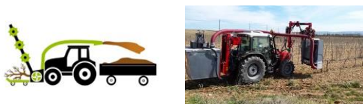
Figure 5: Vineyard pre-pruning integrated with collection and mulching/chipping (left). Prototype developed by the Vinyards4heat project (right).
