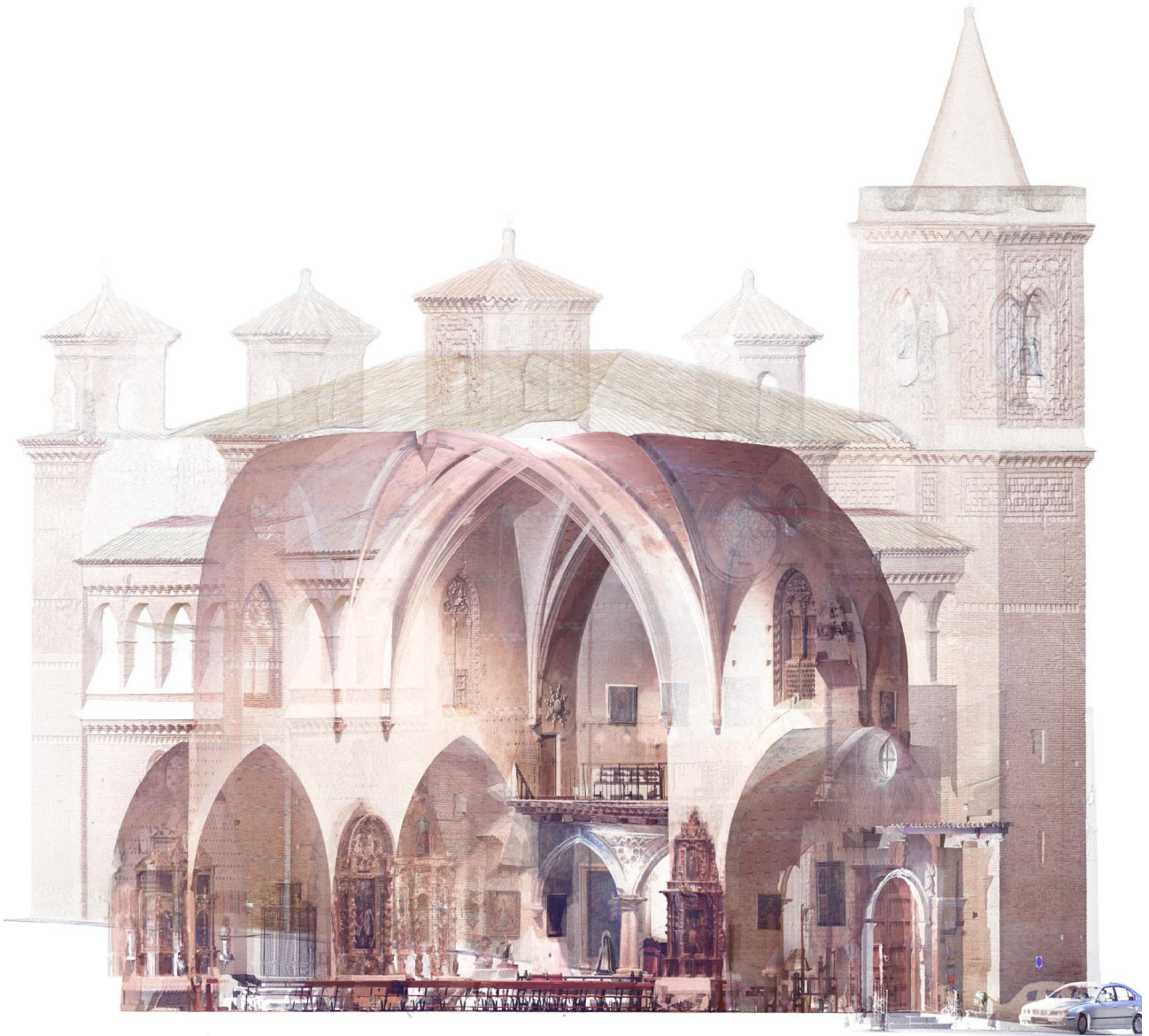
Fig. 9. View sectioned by the arch of the ribbed vault of the digital model. Own elaboration.
