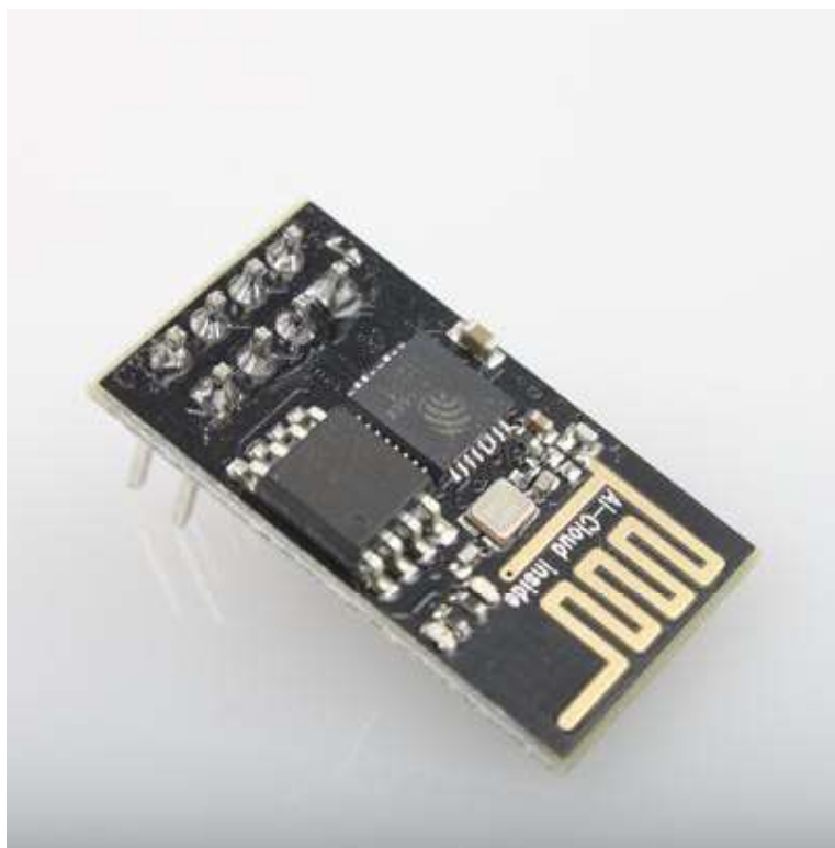
Figure 3 [Module Pin Counts, 8 pin, 14.3 mm *24.8 mm *3.0 mm]
