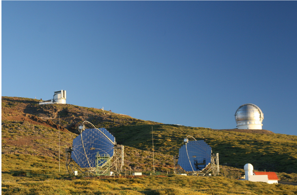
Figure 4.1: Picture of the MAGIC telescopes, MAGIC I on the left and MAGIC II on the right. On the lower right corner, the Counting House (CH) building is seen, from where the telescopes are operated. Above the MAGIC telescopes appear, the 3.5 m Galileo telescope (left side) and the 10 m GTC telescope (right side), currently the biggest optical telescope worldwide. Credit: Dr P.Peñil.
