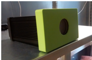
Figure A.37: Picture of the light flasher used for testing the calibrations.
