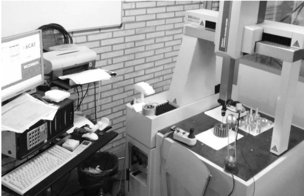
Figure 34. CMM (from the room camera) used in the Spanish laboratory to measure a gear.
