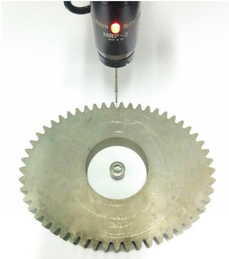
Figure 33. Validation of the algorithm with a coordinate measuring machine.
