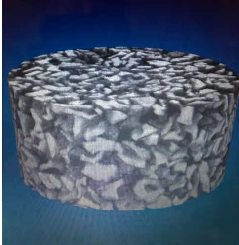
Fig. 5: Micro-CT images of the structure of the particulate graft with a resolution of 11.8 pixels, a scanning time of 3 hours and an exposure time of 8500 ms.
