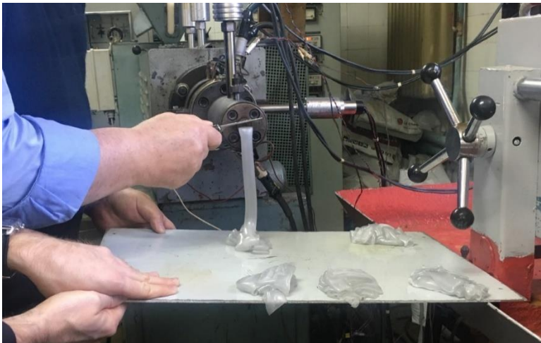
Figure 23. Samples for the measurement of the mass flow
