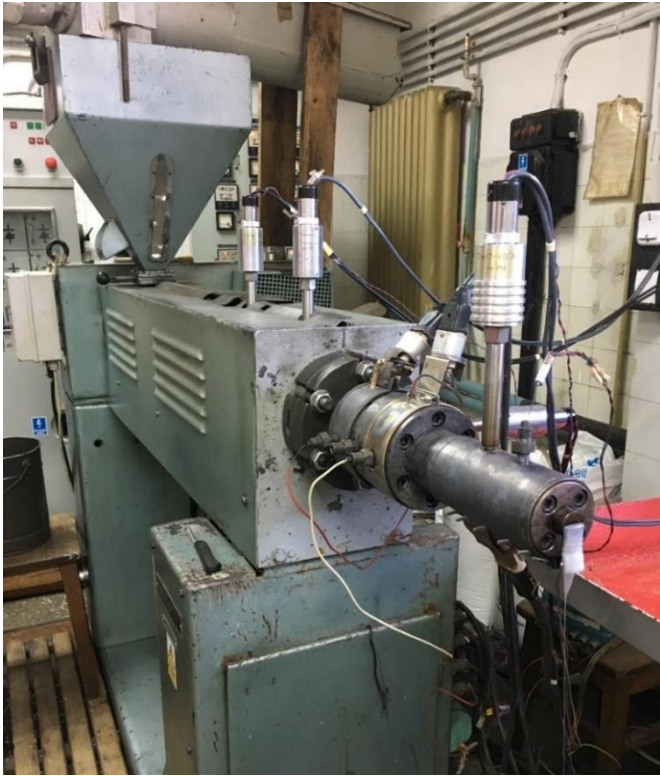
Figure 16. Extruder used for doing the experiments
