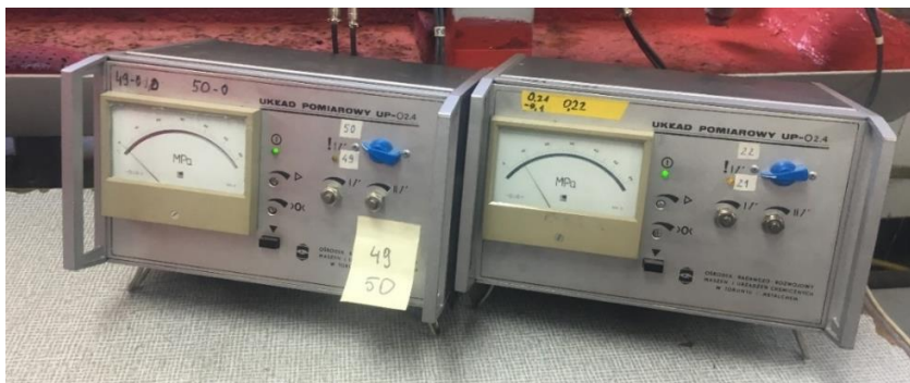
Figure 20. Devices used to measure the pressure
