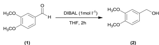
Figure 1: Step 1 of the synthesis procedure of (±)-DMBO. Reduction of 3,4-dimethoxybenzaldehyde (1) to 3,4-dimethoxybenzyl alcohol (2).
