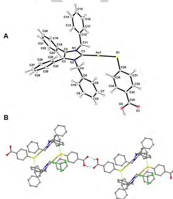
**Figure 3.** A. ORTEP view of the molecular structure of **1a** showing the labelling scheme. The labels for hydrogen and some carbon atoms are omitted for clarity. B. Crystal packing of **1a**·CHCl<sub>3</sub> showing the intermolecular contacts. The supramolecular packing is formed by hydrogen bonds (light blue lines) ( $1.782\text{ \AA}$ ), S...H<sub>CHCl<sub>3</sub></sub> ( $2.534\text{ \AA}$ ) and S...H<sub>Ph</sub> ( $2.874\text{ \AA}$ ) (green lines) interactions.
