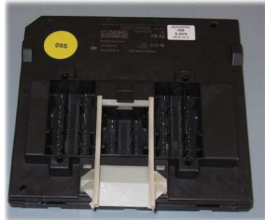
5.a onboard supply control unit (located under the dashboard)
