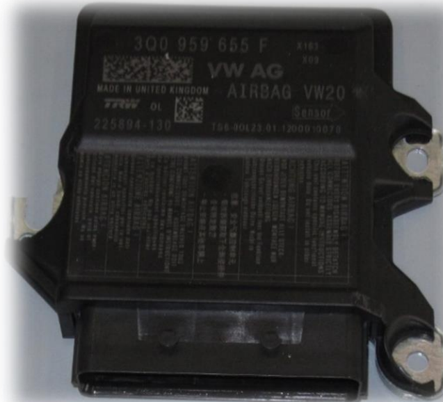
16.b airbag unit (located under the dashboard)
