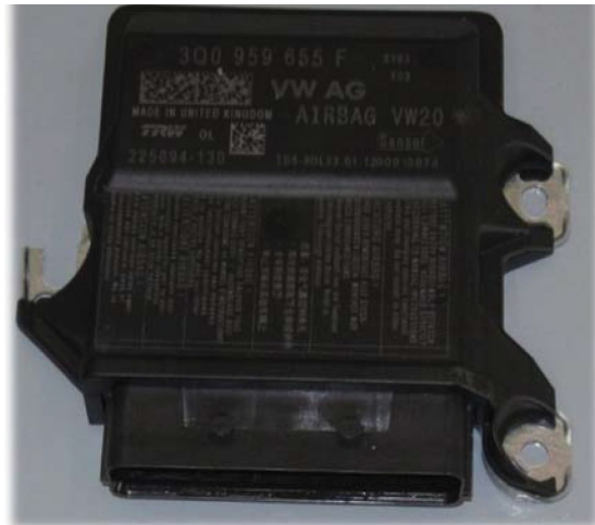
5.b airbag unit (located under the dashboard)
