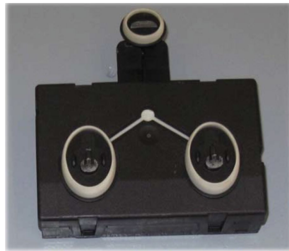
5.c door control unit (located in doors)
