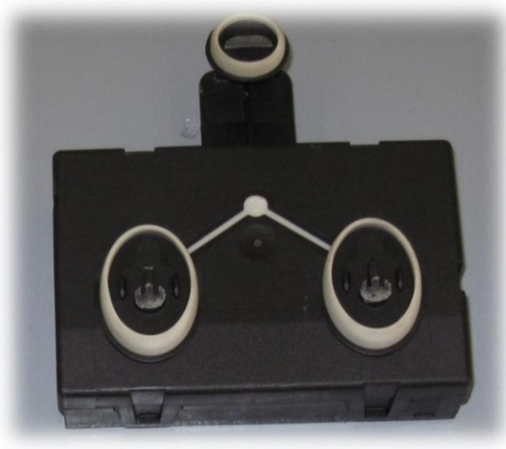
16.c door control unit (located in doors)
