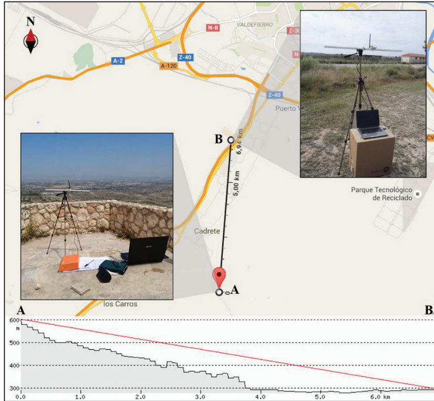
Fig. 1. Distance between both test points and its topographic profile. Point A represents the transmitter station at a vantage point and point B the receiver station at ground level.
