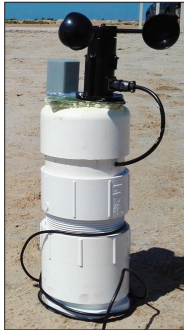
Figure 10. Upper part of the buoy where the electronics are housed and the external sensors are fixed.
