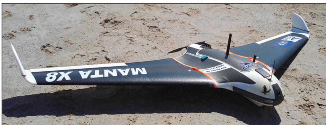
Figure 11. Delta Wing UAV used in the SIMMA project.
