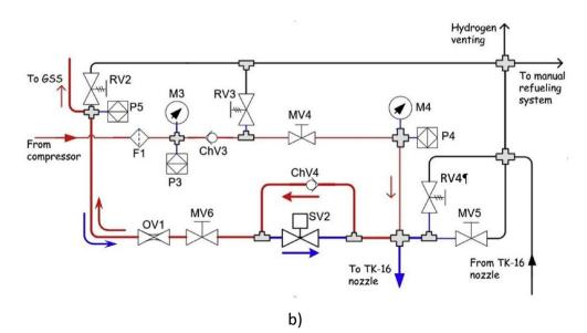
Fig. 7. Panel used to refill the stationary GSS and to refuel hydrogen to the FCHEV.
