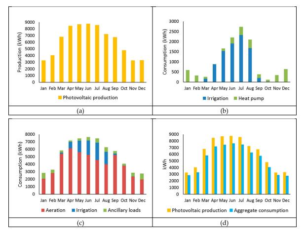
**Figure 14.** Photovoltaic production vs aggregate consumption: (a) Photovoltaic production; (b) Aggregate consumption of the aerators, sludge pumps, and heat pump; (c) Aggregate consumption of all loads, excluding the hydrogen production; (d) Photovoltaic production vs aggregate consumption, excluding the hydrogen production.
