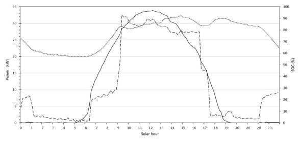
Fig. 10. Electric performance during July 28th, 2017, a day within the irrigation season. The legend is the same as in Fig. 9.
