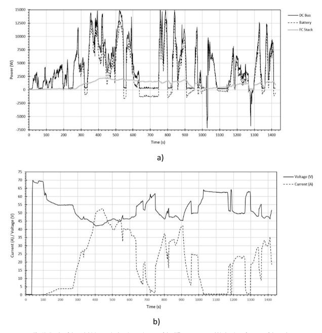
Fig. 12. Results of the real driving test in the winery: a) power of the different sources, and b) electric performance of the stack.
