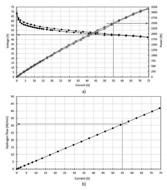
Fig. 7 – Polarization curve (a) and hydrogen consumption (b) of the H-3000 with the hydrogen recirculating system for the nominal operating point (2.5 kW).
