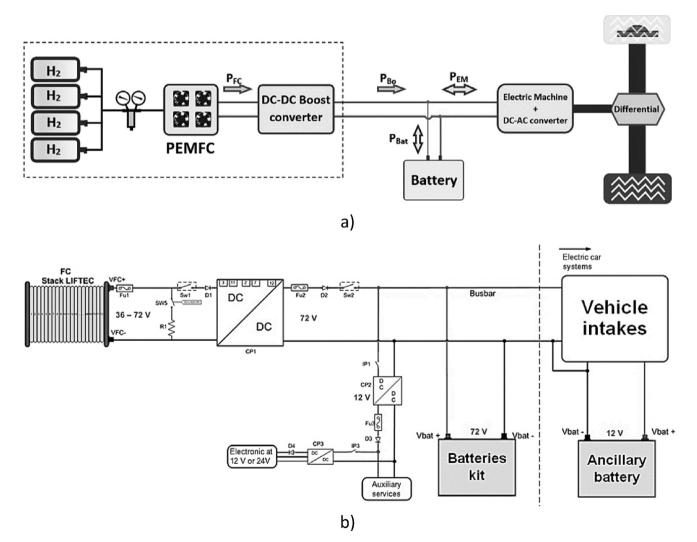
Fig. 5 – Hybrid powerplant of the FCHEV: (a) diagram of the final configuration with the added  $H_2$ +PEMFC system (dashed square); (b) electrical layout.
