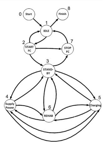
Fig. 6 – Diagram of the operating modes of the state machine used to control the stack performance.
