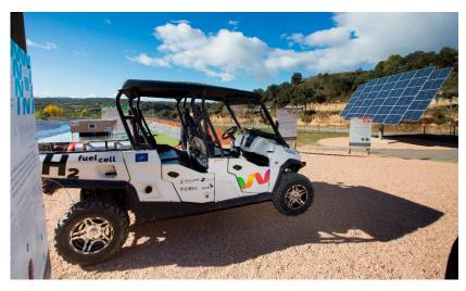
Figure 9. The fuel cell hybrid electric vehicle (FCHEV).
