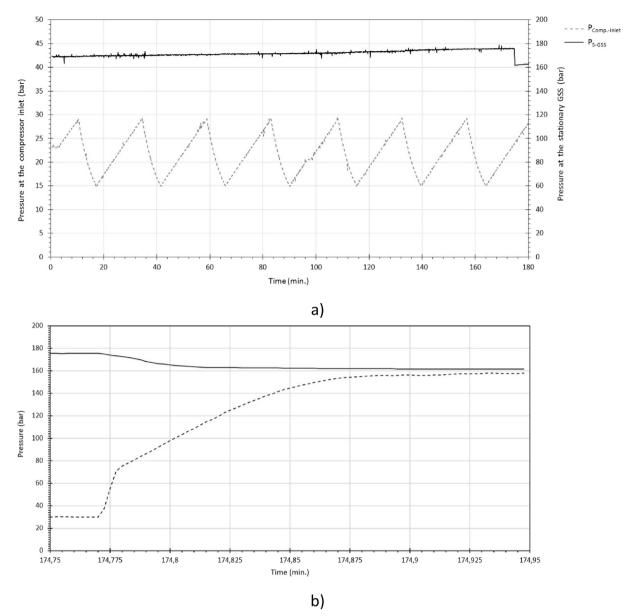
Fig. 11. Performance of both the system to refill hydrogen to the stationary GSS (a), and that to refuel hydrogen to the GSS of the FCHEV (b).
