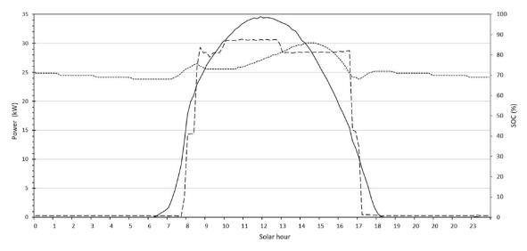
Fig. 9. Electric performance during March 19th<sup>.</sup> 2017, a day out of the irrigation season. Solid line for power production, dashed for consumption, and dotted one for the SOC of the battery bank.
