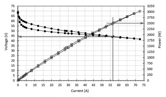
Fig. 3 - Initial polarization curve obtained for the H-3000 in the test bench.
