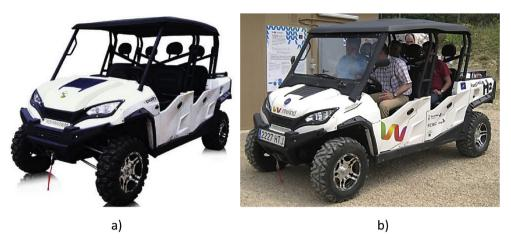
Fig. 8. The original ePath 7500 BEV (a), and the remodeled FCHEV (b).
