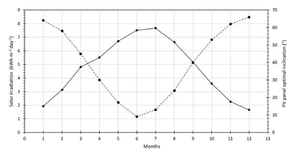
Fig. 2. Estimated values of solar irradiation (solid line) and optimal panel inclination (dashed line) for each month at the winery area [25].
