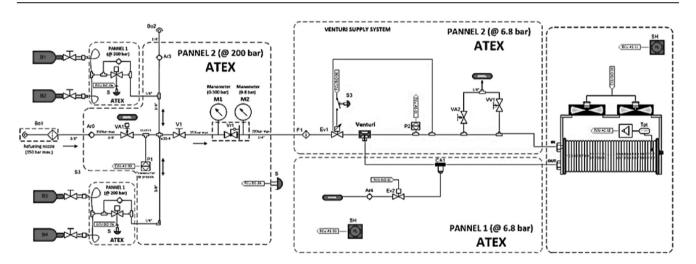
Fig. 4 - Piping and elements diagram of the hydrogen storage and supply system.
