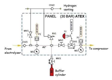
Fig. 6. Panel used to control the correct performance of the compression stage.
