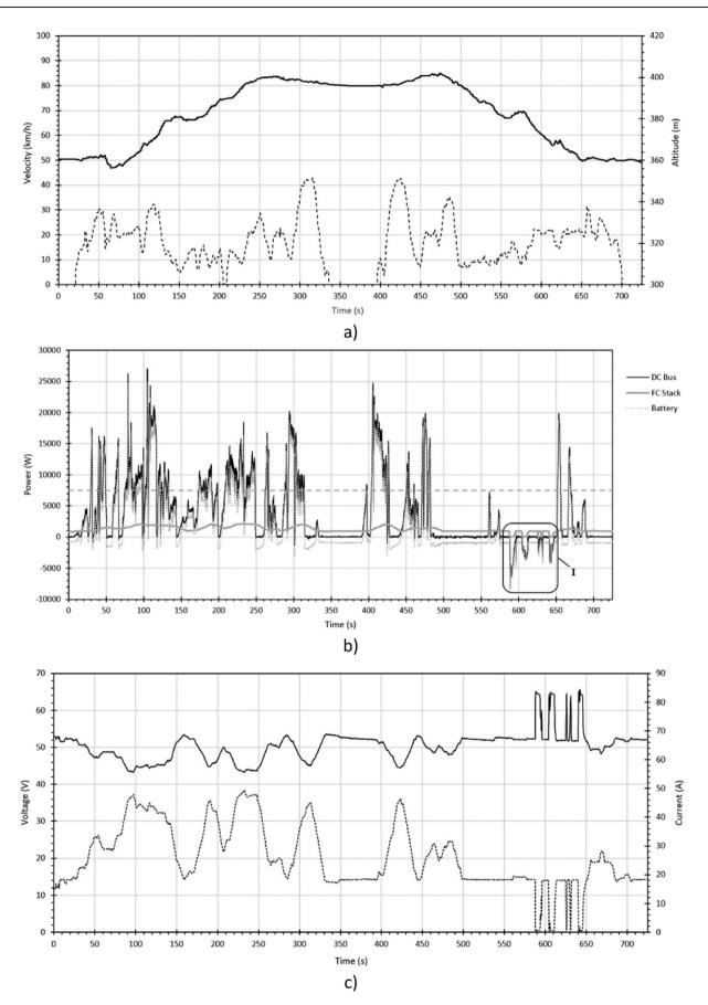
Fig. 9 – Results of the real driving test in the winery: (a) Altitude (solid line) and velocity profiles (dotted line), b) Power of the different sources, and c) Electric performance of the stack (voltage in solid line and current in dotted one).
