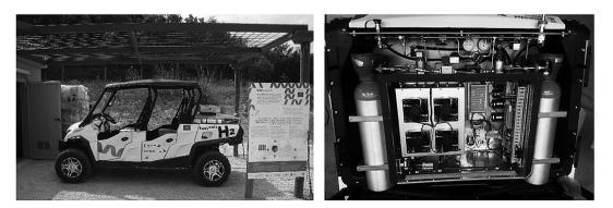
Fig. 2 – Two photos of the modified electric car with the  $H_2$ +PEMFC system assembled at the rear platform.
