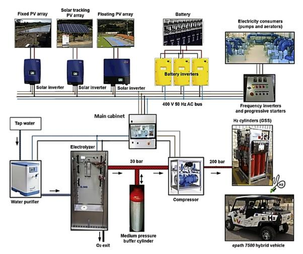
Fig. 1. General scheme of the power-to-gas plant of this project.
