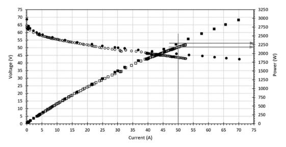
Fig. 8 – Comparison of the performance of the PEMFC stack: Initial (solid symbols) vs. 1000 h at the winery operating conditions (empty symbols).
