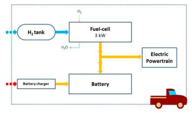
Figure 10. Block diagram of the FCHEV.
