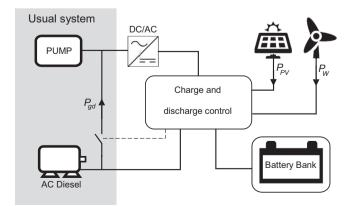
Fig. 1. Proposed hybrid power system.
