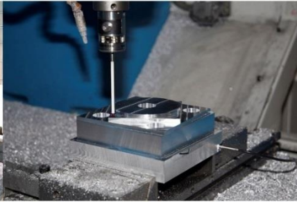
Figure 2-1 On-MT measurement experimental exercise: a) Workpiece manufacturing scenario; and b) on-MT measurement with RENISHAW OMP 400 tactile probe. [176]
