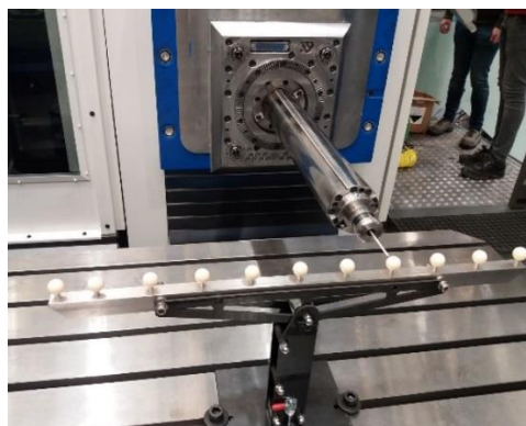
Figure 1-10 Artefact measurement-based MT characterisation.
