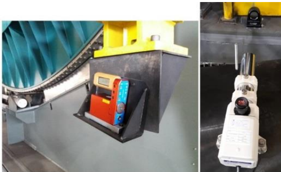
Figure 12. Direct measurement methods for the pointing repeatability test.
