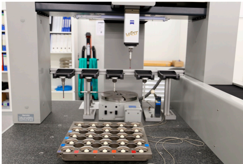
Figure 9. 3D artifact for CMM error characterization.
