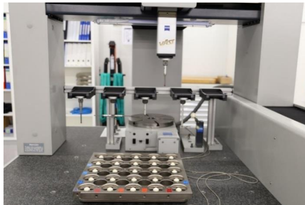
Figure 1-9 3D artefact for VCMM characterisation. (Zeiss UPMC Carat 850 CMM at IK4-TEKNIKER premises). [6]
