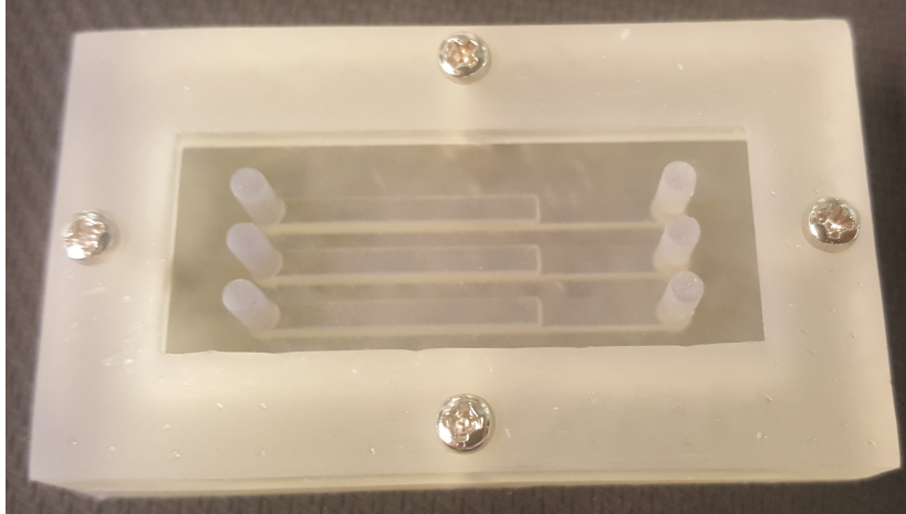
Figure 2.13: Final mould made of a biocompatible resin by stereolithography, used for the fabrication of the final devices
