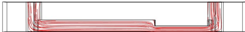
Figure 2.6: Streamlines in the longitudinal section of the final geometry. The possible flow disturbance due to the presence of the inverse step would not affect the cells seeded. Flow direction is from left to right
