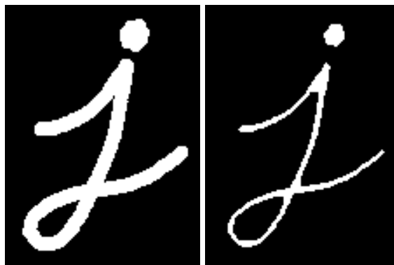
Figure 2.5: Erosion example. Source: OpenCV [10]
