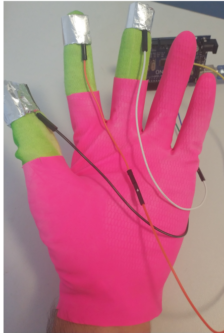
(c) Connection of the Arduino pins to the rings in the hand.
