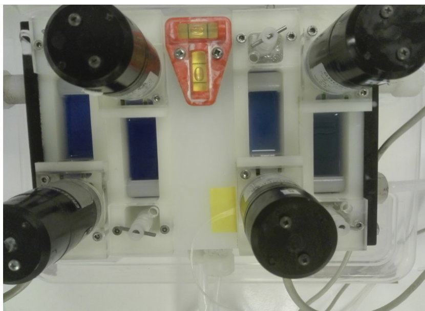
Figure 12: Mixer settlers system with 2 extraction and 2 stripping stages with NaOH added.
