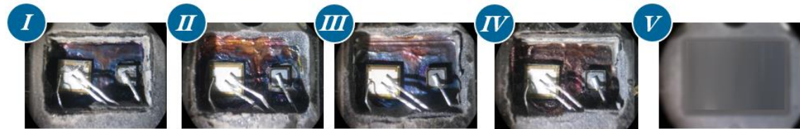
Fig. 5.2-6. Measured devices with the IGBT and diode chips visually accessible (devices I to IV) and a closed device used for reference (device V).
